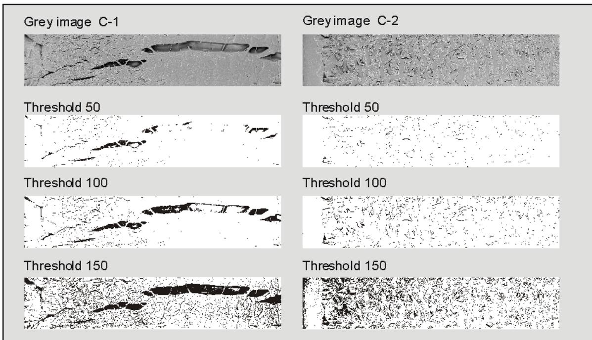
Figure 3 Thresholding of grey images
